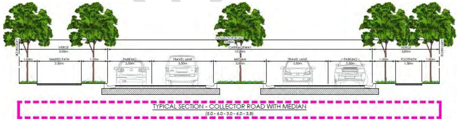
Figure 13: Collector Road with Median
