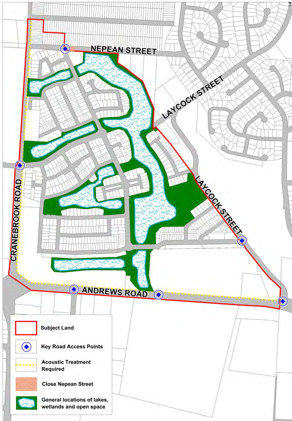
Figure 12: Key design elements (Waterside Residential)
